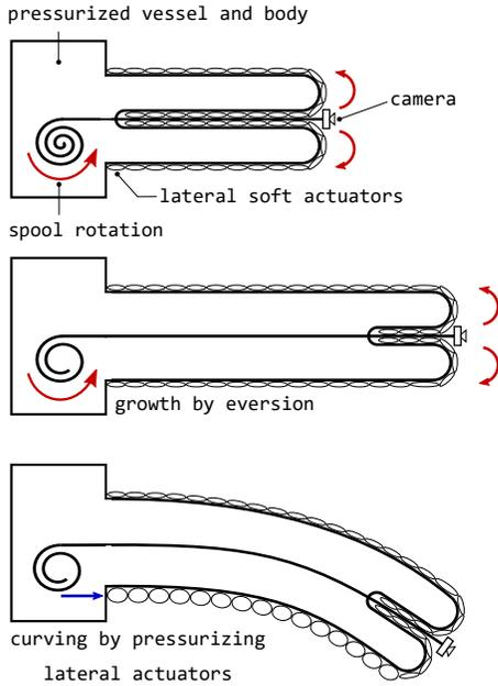
Fig. 1. The concept of growth by eversion of material rolled onto a spool and the concept of curving by pressurization (and thus, contraction) of actuators placed and sealed on the main body.
