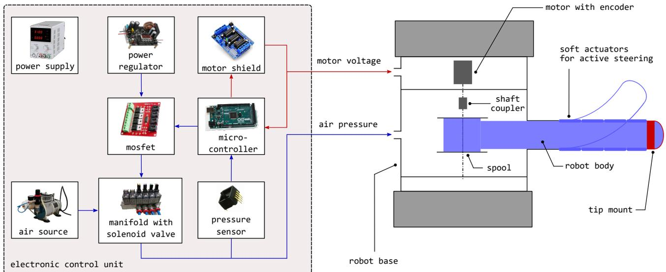
Fig. 3. Architecture of the proposed soft growing robotic system (*dimensions not to scale*).
